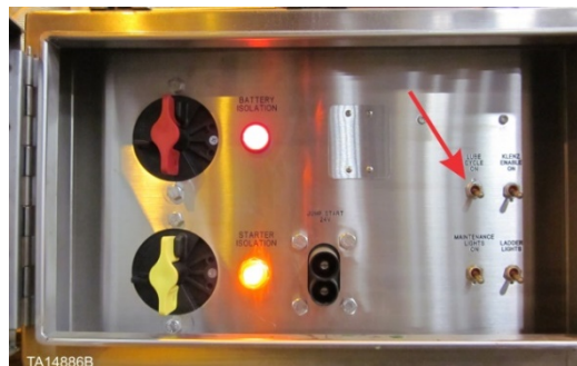
Lubrication cycle switch inside control switch box located on left rear of machine
