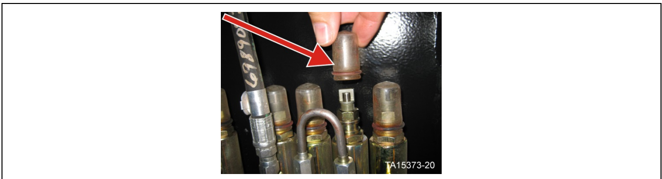
Figure 59. Install the plastic caps to protect the injectors from contamination
