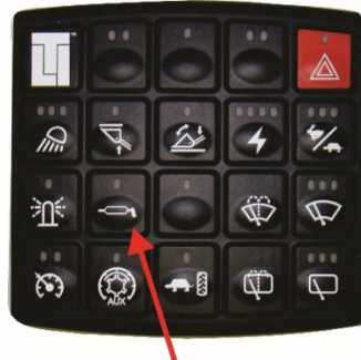
Lubrication switch on overhead panel in operator cab
