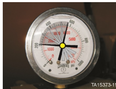
Figure 32. Pressure gauge with pump speed too fast wide swing in pressure (cavitation occurs)
